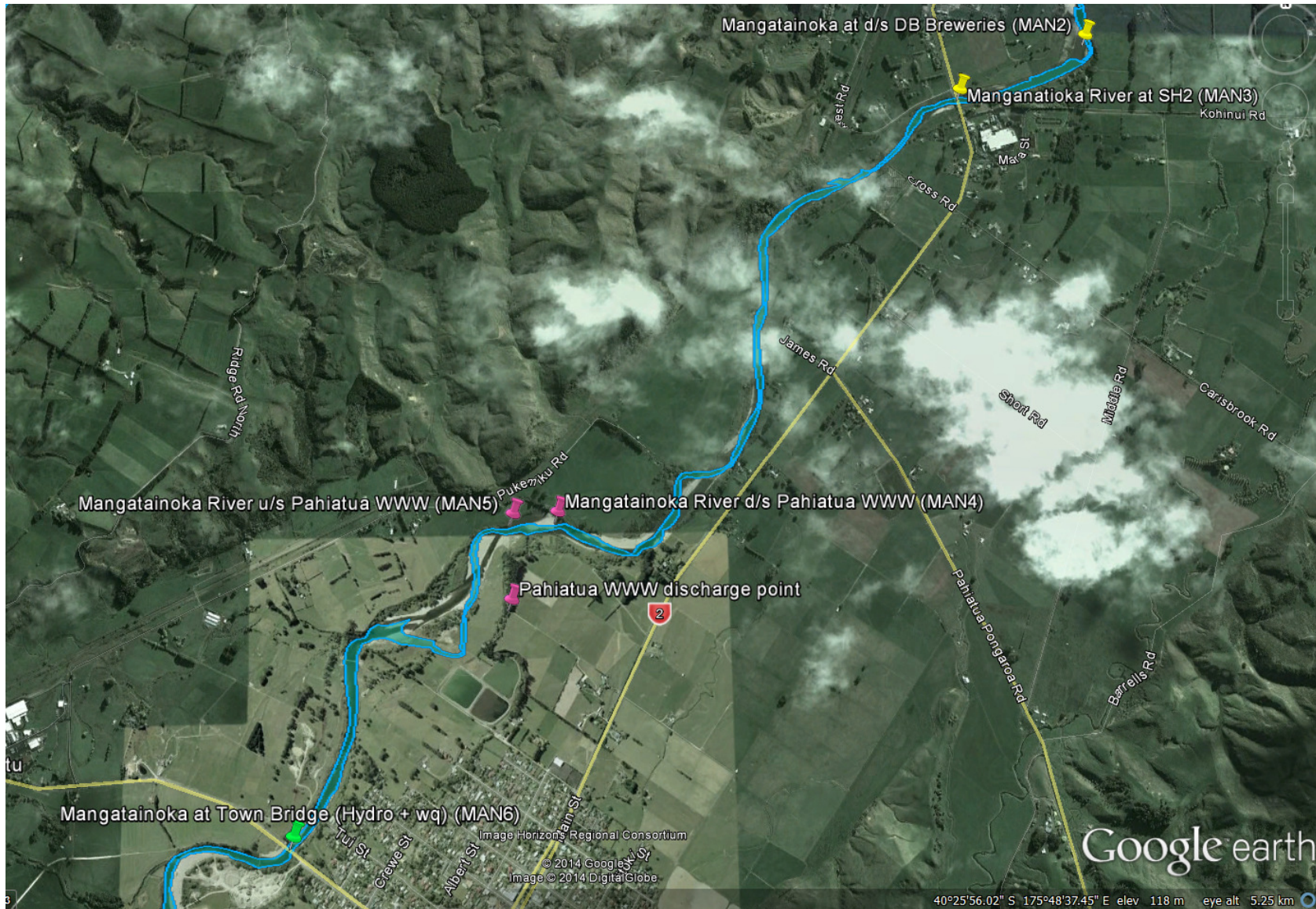
Figure 3. Location of water quality sampling points closely related to the wastewater discharge and Town Bridge hydrometric monitoring station
