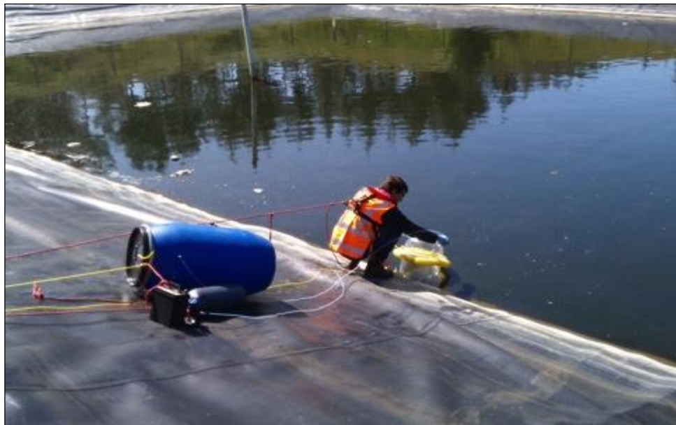
Figure 2.1 : Preparing the flux chamber for sampling at the edge of the leachate pond
