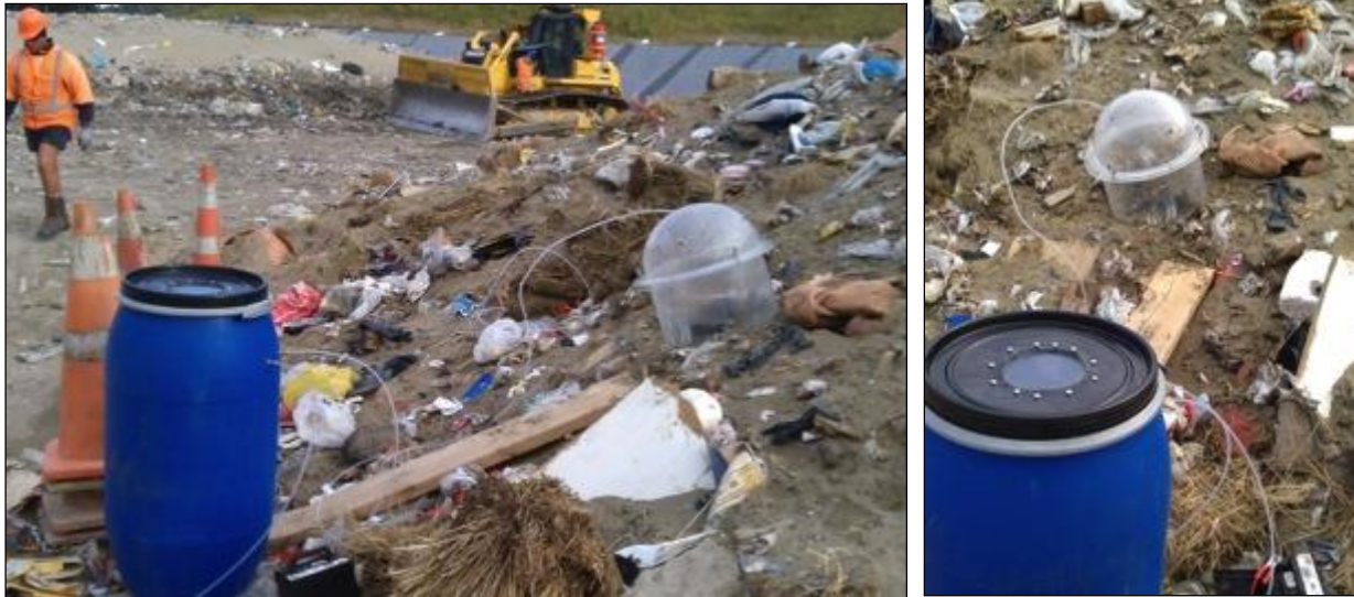
Figures 4.7 depicting the location of sample site four on the active tip face while Figure 4.8 reveals the refuse upon which the flux hood was sampling.
