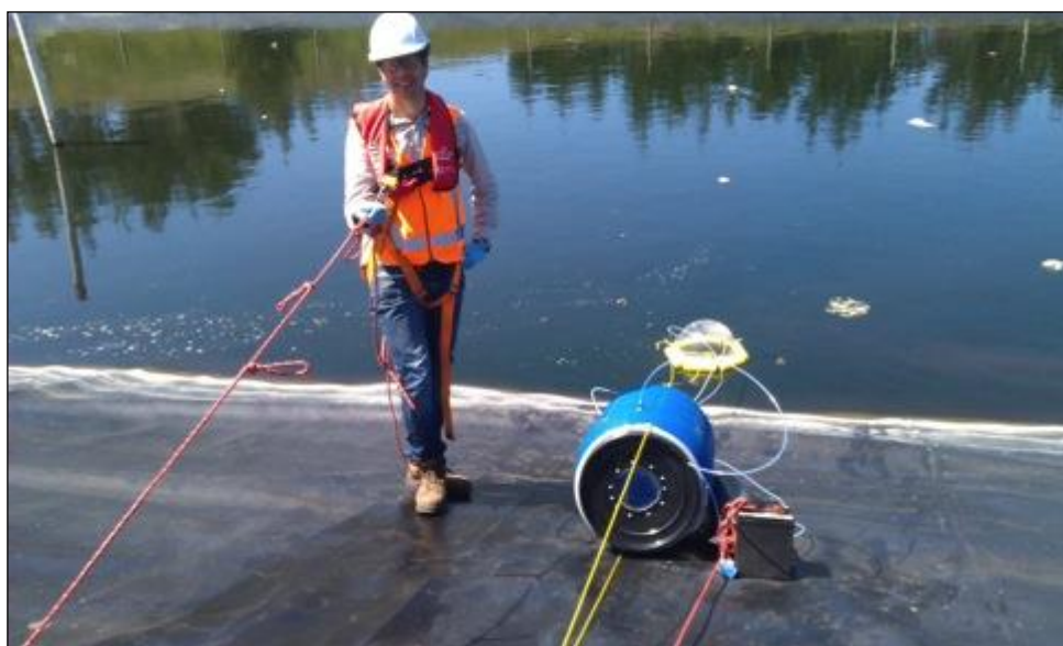
Figure 2.2 Sampling the Leachate pond. Minimal pond scum was evident during the sampling.
