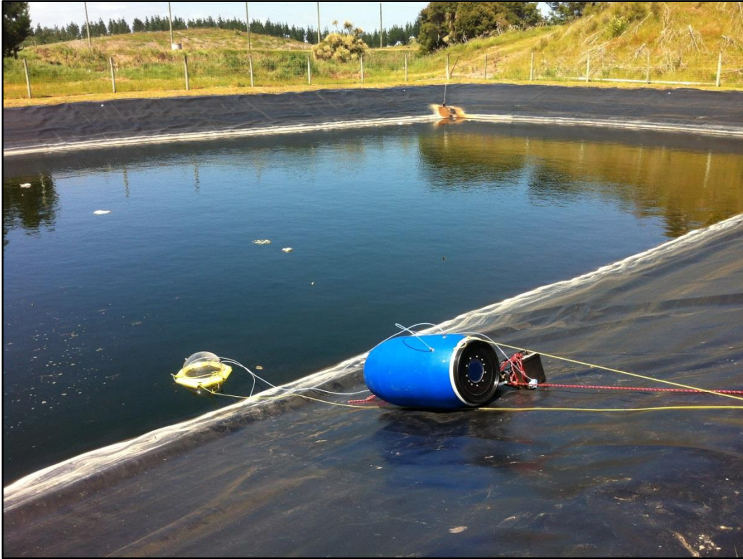
Figure C-3: Photo Looking South-West Showing Odour Monitoring at the Leachate Pond
