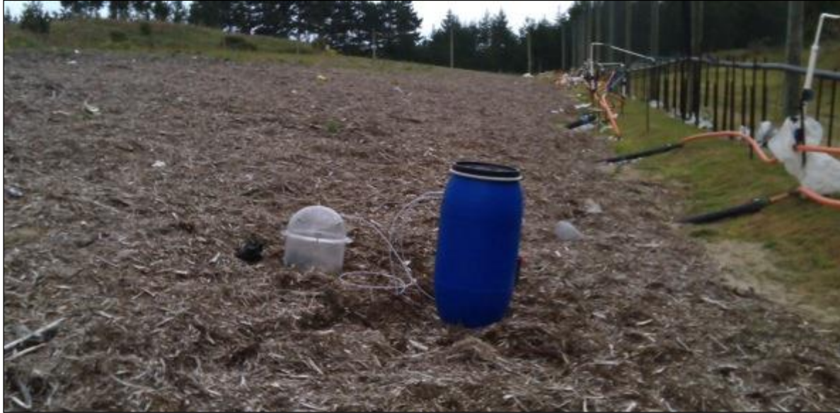
Figure 5.1 Sampling of the gas discharge identified during the walkover survey the preceding day.
