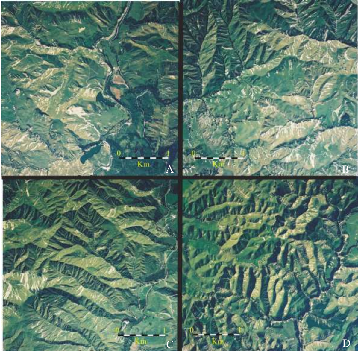
Figure 23. Four vertical aerial photos used for landslide counts in different study areas: A - Mangawhero, B - Whangaehu, C - Turakina, D – Pohangina ( original print scale 1:18 000 ). These photos clearly show the differing landslide densities and styles of landsliding in the four areas. Note that the very large (~100 million m 3 ) prehistoric Otoko Lakes landslide (bottom right, A) was unaffected by the rainstorm, as were many other very large prehistoric landslides in the region.
