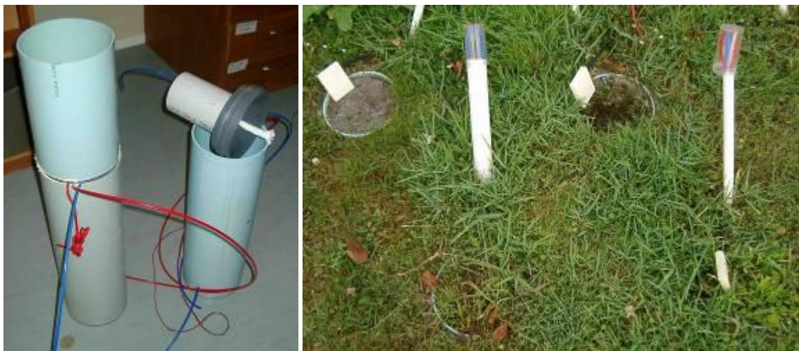
Figure A9. The three types of fluxmeters used by van der Velde et al. (2005) on Tongatapu to monitor the losses of nutrients and pesticides to groundwater
