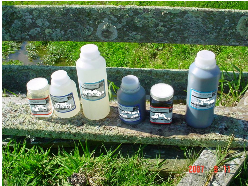
Samples taken by officer in relation to the photograph above – the 3 samples on the left from upstream and those on the right are from effluent being discharged.
