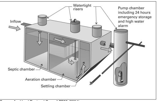
Figure 4.2 Example of an Aerated Wastewater Treatment System
