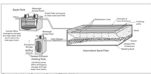
Figure 4.3 Example Of An intermittent Sand Filter
