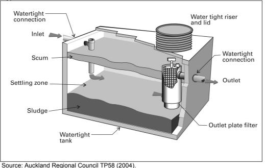
Type B. Plate Disc Dam Effluent Outlet Filter
