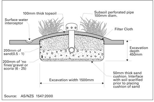
Figure 6.5 Typical Evapotranspiration Seepage Bed Detail
