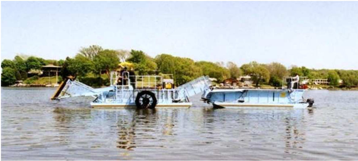
Figure 2-9: Weed harvester. Small weed harvester (left) is driven by paddle wheels with a cutting speed of 2 to 4 km/h – cutter assembly at front (left). It has a hold capacity of up to 10 t wet weed (depending on model). The unloading conveyor ramp at the back can off-load to a truck at the landing or into a transport barge (right) to allow it to continue working while the transport barge shuttles the weed to shore. Generic photo from web.
