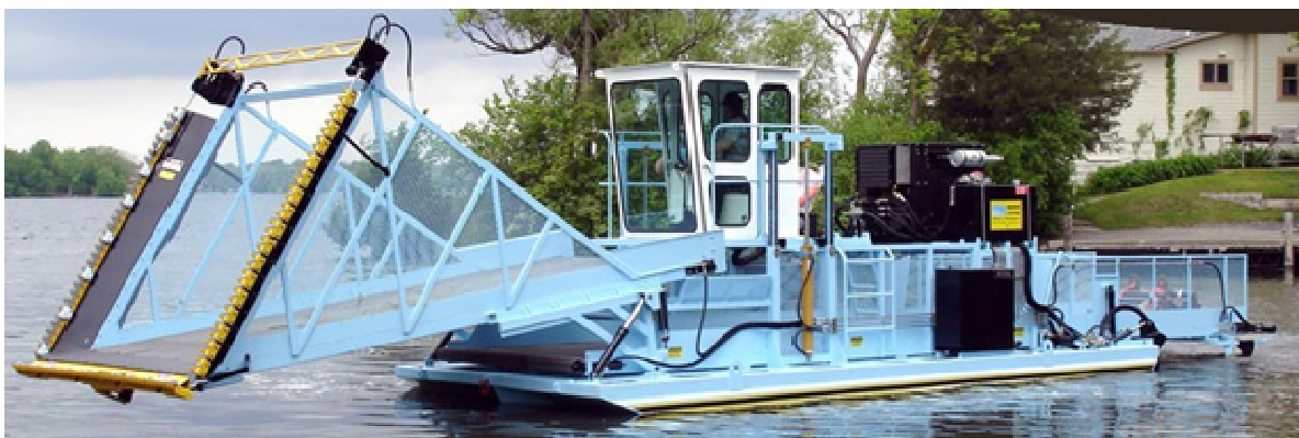
Figure 2-10: Weed harvester cutters. The cutter blades are about 2 m long on both sides and across the bottom with the cutter head able to be raised and lowered to adjust the cutting depth. The ramp behind the blades draws the cut weed into the hold of the harvester. This image shows a harvester without the paddle wheels attached, as would be needed for road transport. (Generic photo from the web).
