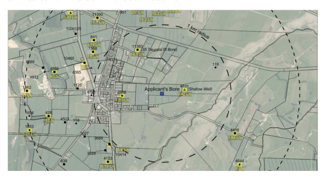
The effects of your proposed take on groundwater levels in neighbouring bores needs to be assessed. Each pumping bore will draw water from the surrounding aquifer, resulting in a drop in pressure in a confined aquifer, or a reduction in the water table in an unconfined aquifer. This is known as the drawdown or 'interference effect', where it has a measureable effect on other bores.
