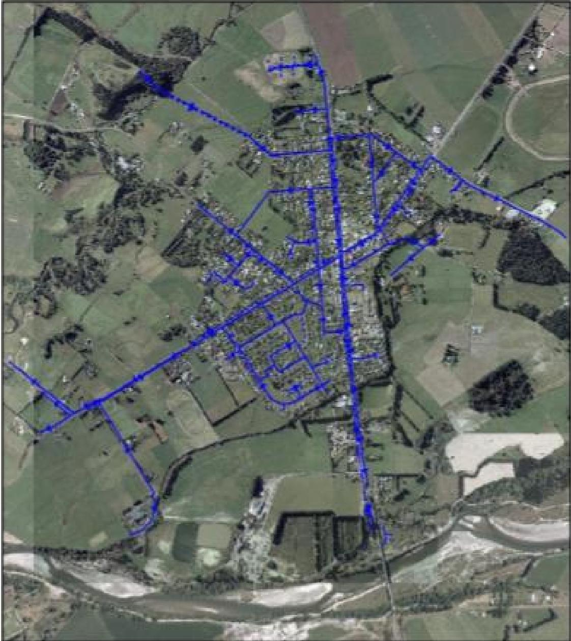
Figure 2.3: Water Reticulation Network (from Rangitikei District Council Asset Management Plan 3 Waters, 2014)
