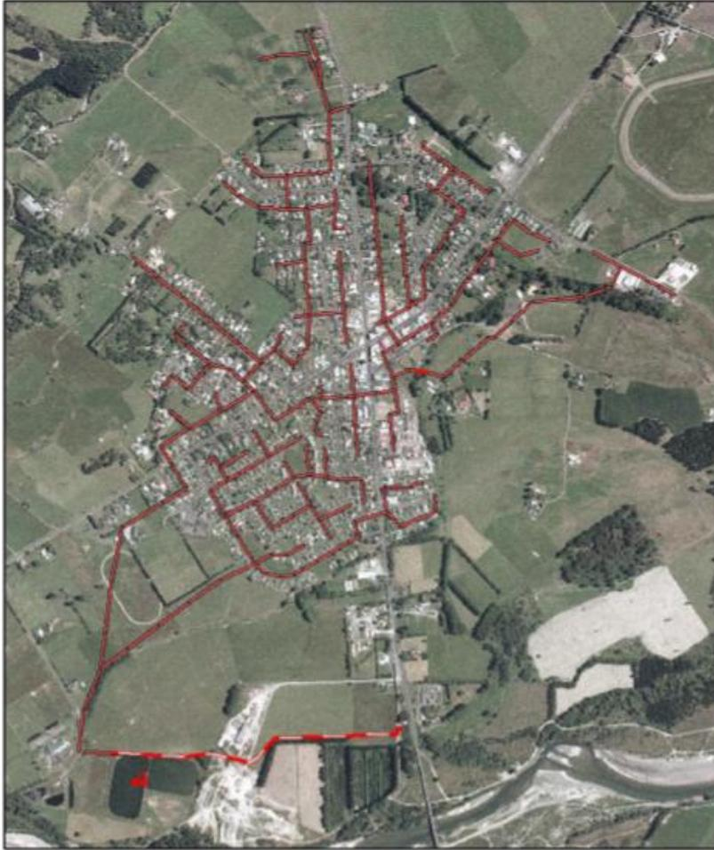
Figure 3.2: Bulls Waste Water Treatment Scheme Layout (from Rangitikei District Council Asset Management Plan 3 Waters, 2014)
