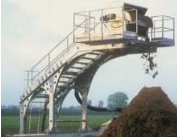
Photo 8. Screw press solids separator.
