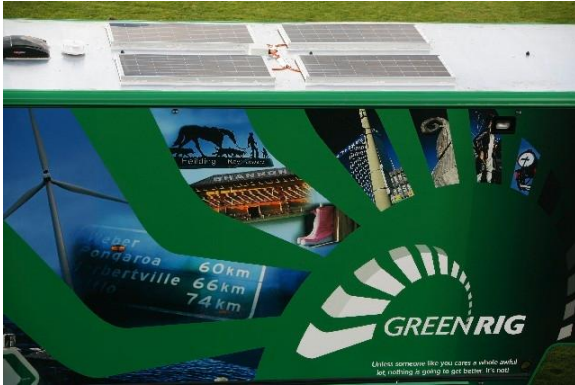
One kilowatt of roof-mounted solar panels
