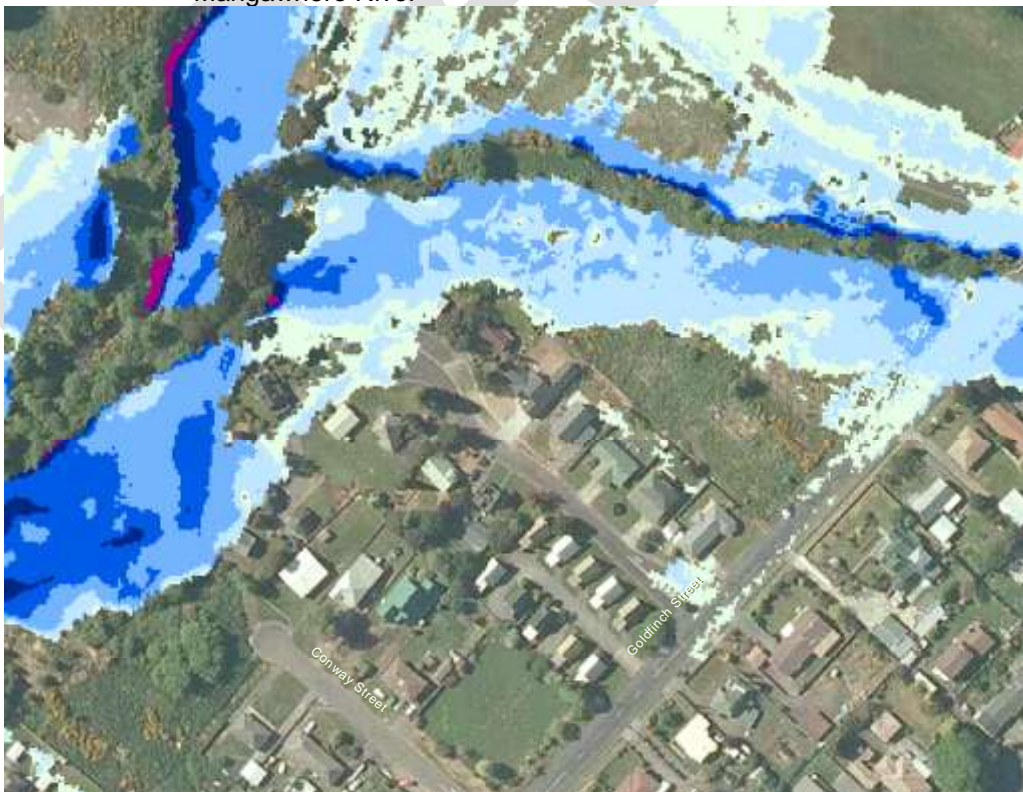
Figure 5.4: Ayr, Rata and Tay Streets and CBD flooding mainly from Channel B overflows
