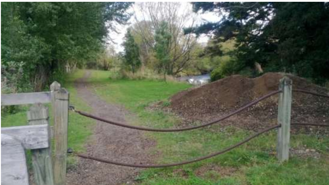
Photo 28: Immediately downstream of Mangawhero Terrace turning circle. The 0.5% AEP flood map indicates there is no stopbank required here. However, there is an overflow path around 60 metres downstream. This may be cut off by the Miro Street Drain stopbank works.
