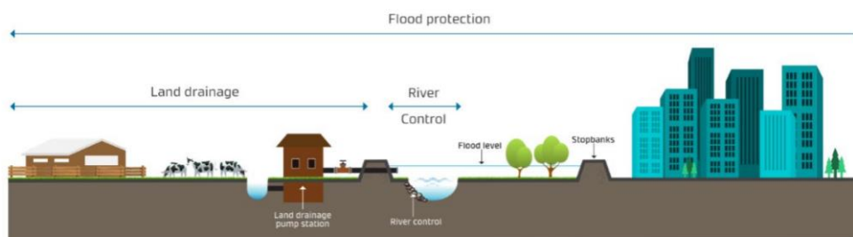
Figure two: Schematic of flood protection scheme and land drainage services (Source: Tonkin and Taylor, March 2018)
