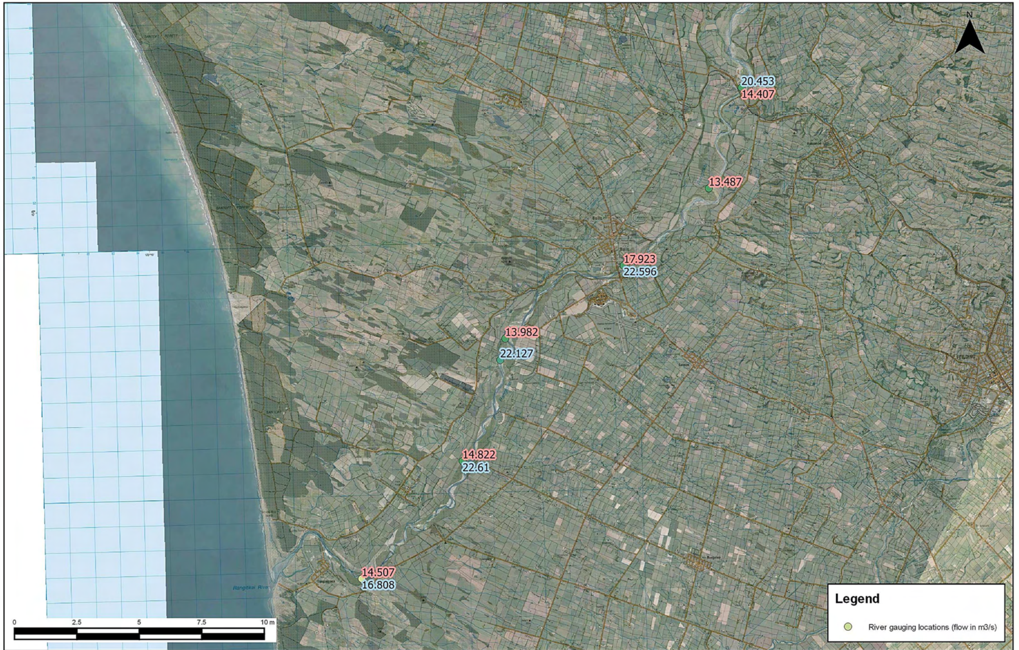
Figure 4.10: River flow gauging locations from Massey University 2015 survey. Values in blue represent flow on 6 January 2015 and values in red represent flow from 20 January 2015
