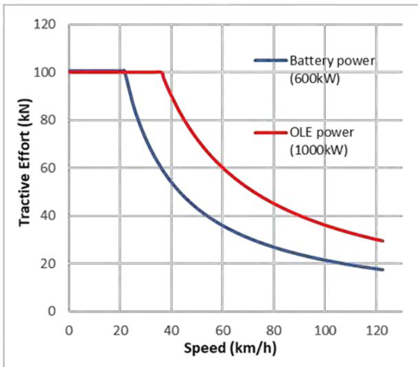
With 600kW available, the train can accelerate as fast in battery mode as it can in OLE mode up to 6m/s (22km/h). Above that speed, the TE falls in inverse proportion to speed. In OLE mode, the TE only starts to reduce after 10m/s (36km/h).
