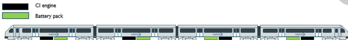
On a B-DMU, a generator/motor is placed within the mechanical drive train between the CI engine and the final drive gearbox. The battery can be charged by running the engine and by regenerative braking. The battery energy can then be used to boost the CI engine or to run the unit for a short distance without the CI engine running.
