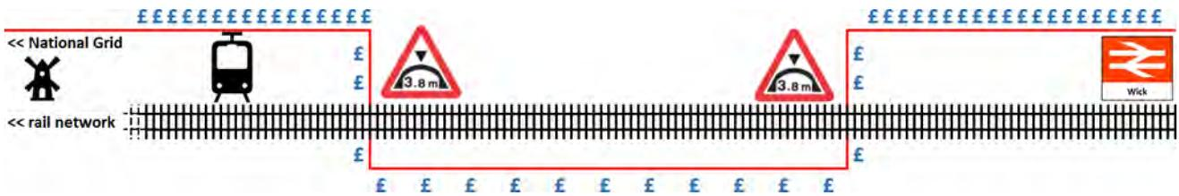
The second scheme shows an alternative approach. In this, the high cost of rebuilding one bridge is justified because it enables the OLE to be run all the way to the second bridge, at which point it ends completely, thus saving the cost of any further OLE and buried cable. This approach is only viable if the trains have sufficient battery autonomy to run the twice the length of the gap (there and back) and run their auxiliary loads for the whole time, including the station dwell time.
