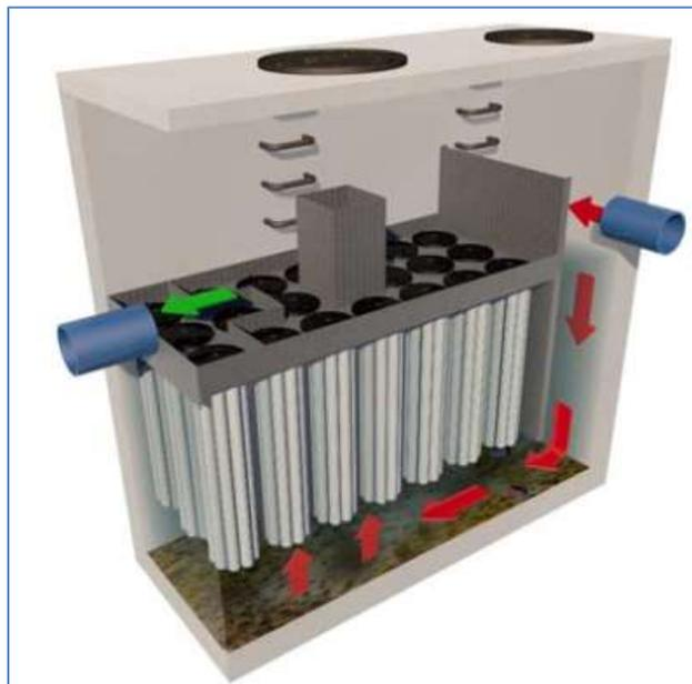
Figure 3.1: Typical Vault Jellyfish filter
