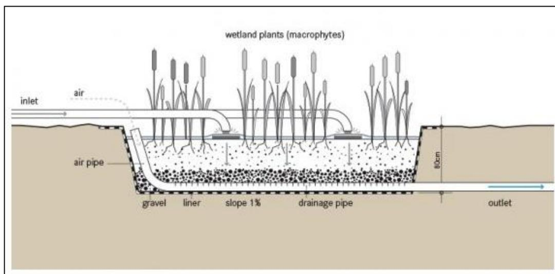
Figure 1: Diagrammatic representation of a Vertical Flow constructed wetland (source Eawag et al 2018).
