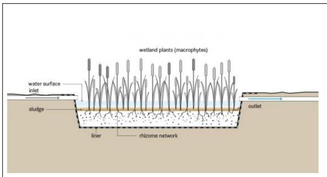
Figure 2: Diagrammatic representation of a Surface Flow constructed wetland.
