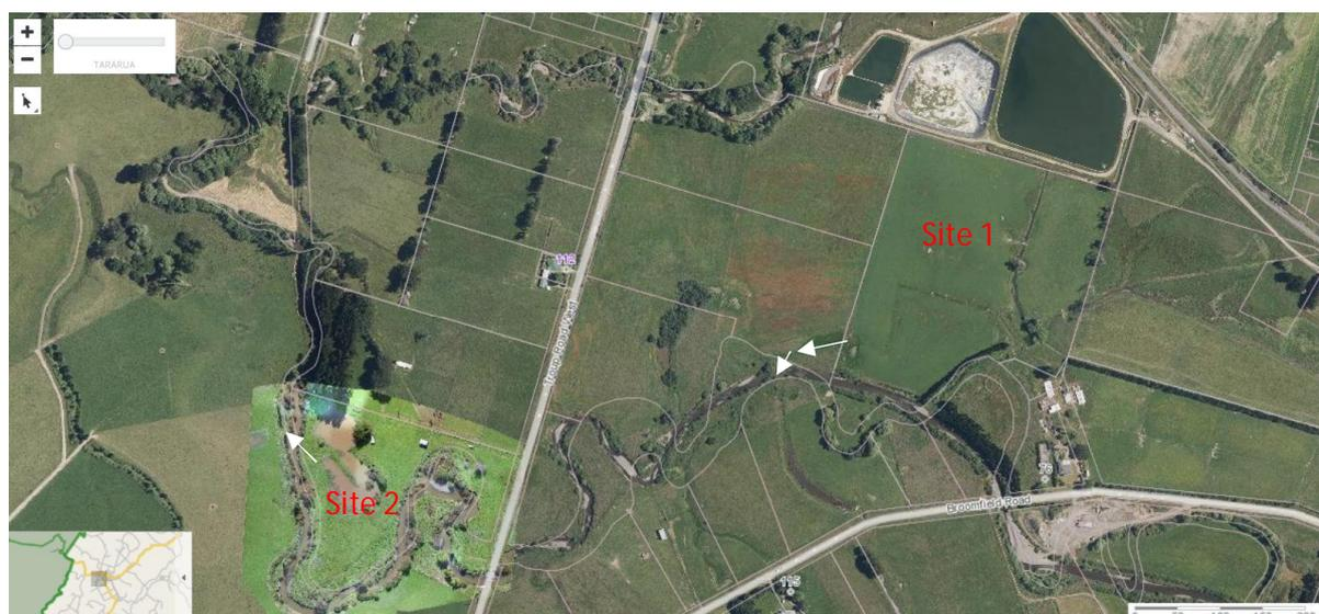
Figure 3: Location of the two wetland site options (white arrows show possible locations for the wetland discharge to the Mangaatua Stream)
