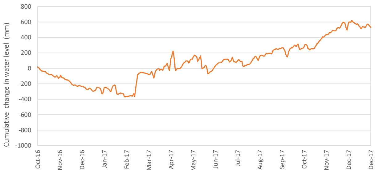
Figure 7: Cumulative change in volume in the treatment ponds, converted to water level (mm) for the period since October 2016.
