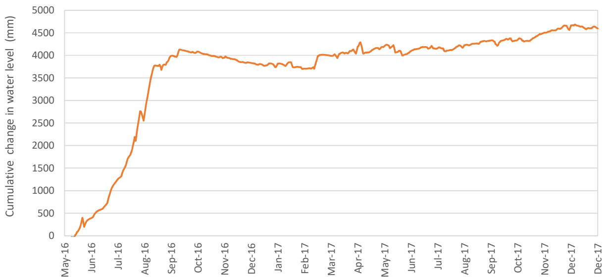
Figure 5: Cumulative change in volume in the treatment ponds, converted to water level (mm).
