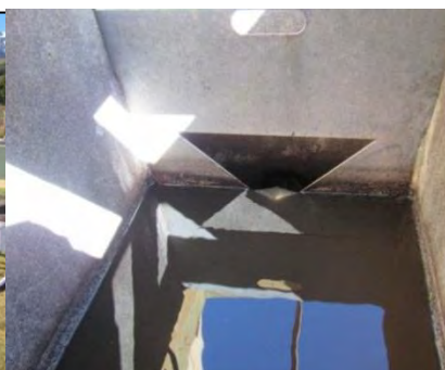
Figure 9 Flow measuring chamber with V-notch weir flow meter
