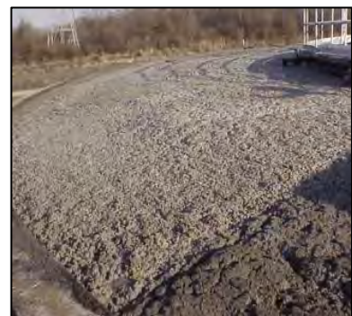
Figure 21 Thick, dark scummy foam
