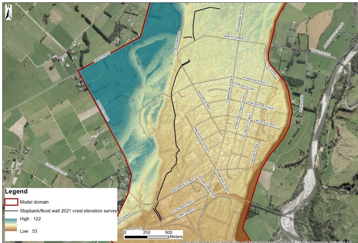
Figure 2.1: Locations where 2021 surveyed stopbank crest elevation data was applied to the model
