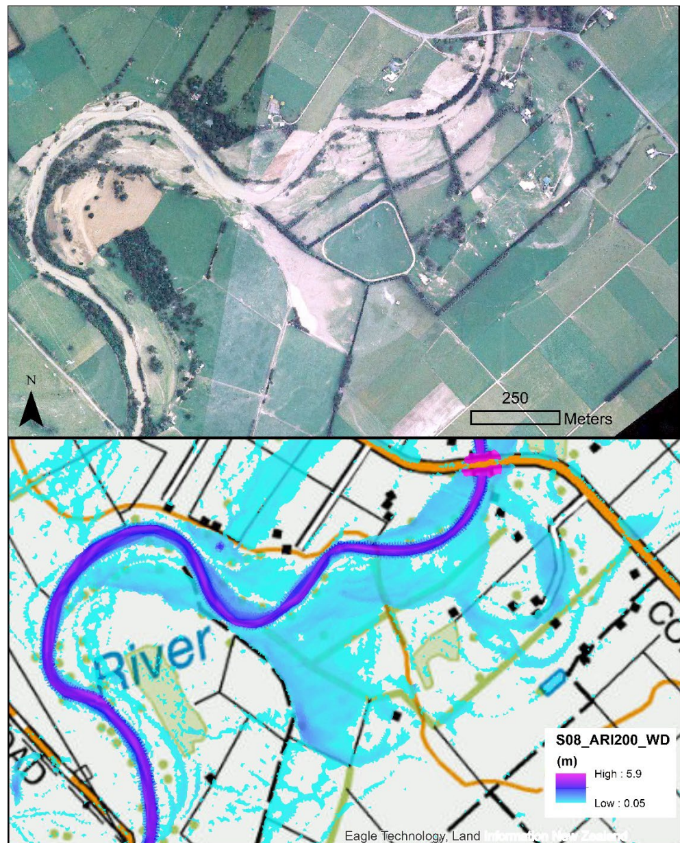
Figure 4-2: Comparison between post-flood aerial photo and model results downstream of Colyton Bridge
