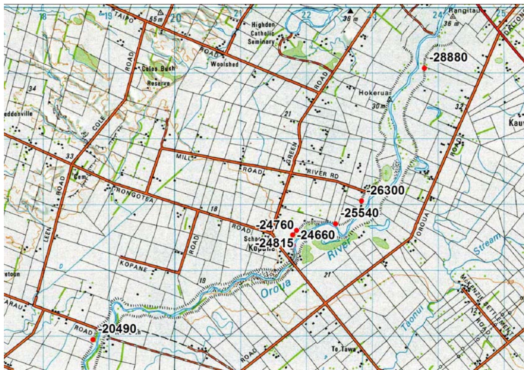
Figure 3-5 Map of the middle Oroua River with stopbank breach locations modelled using MIKE 11 dam-break structures.
