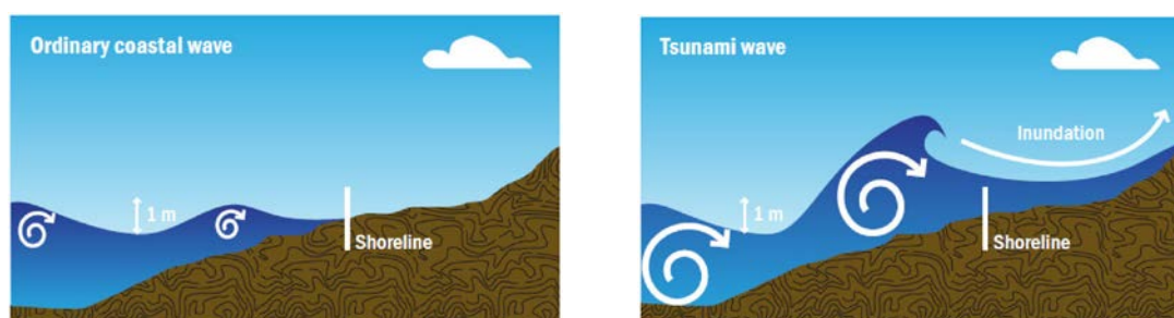
Figure 1 The difference between a coastal wind wave (left) and a tsunami wave (right).
