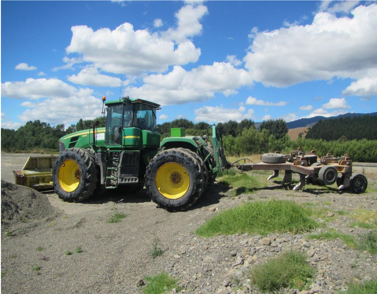
Beach clearing machine with 750mm deep rippers
