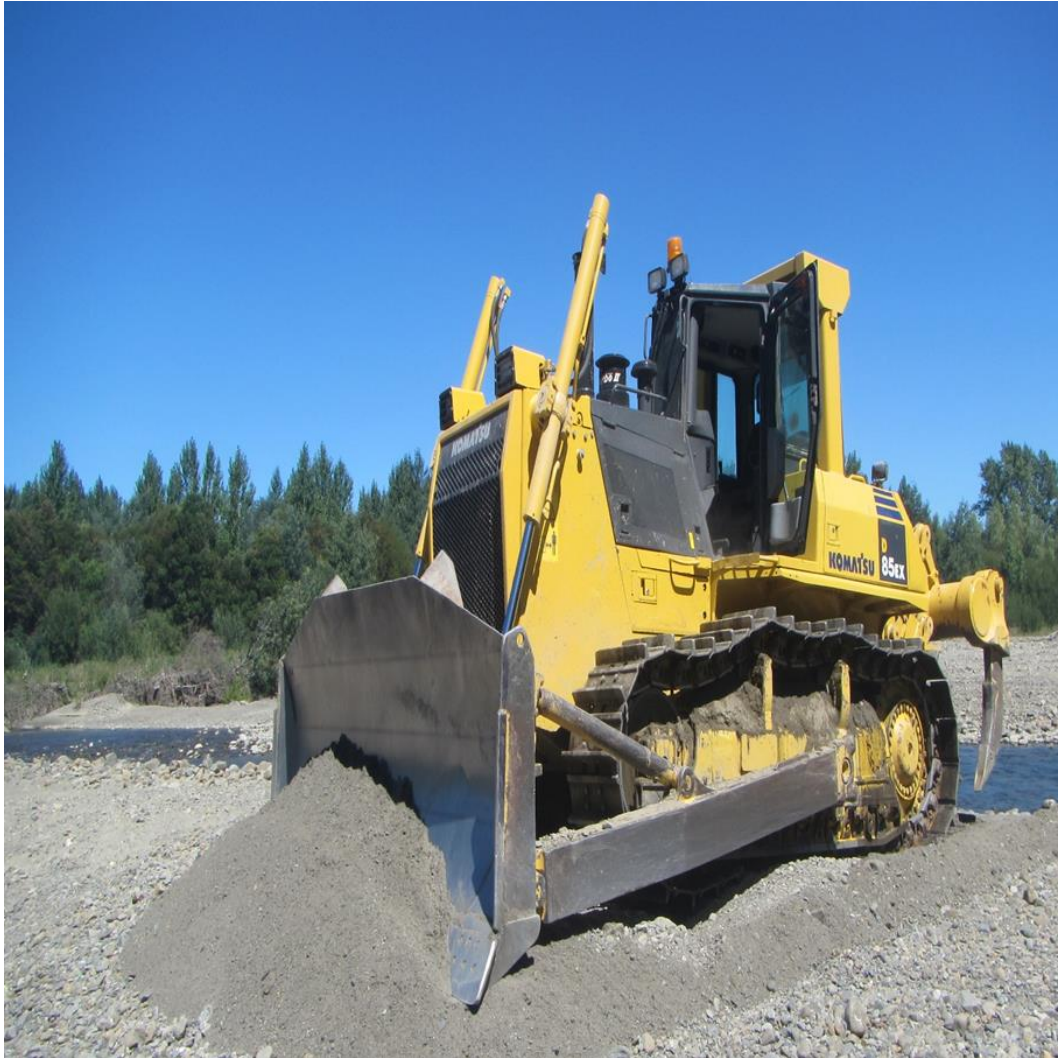
26 Tonne Komatsu Bulldozer on the Pohangina clearing the beaches
