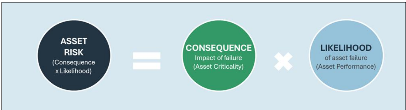
Figure 6: Equation for asset risk (References: ISO 31000 and IAM Risk Assessment and Management, Version 1.1 October 2016).
