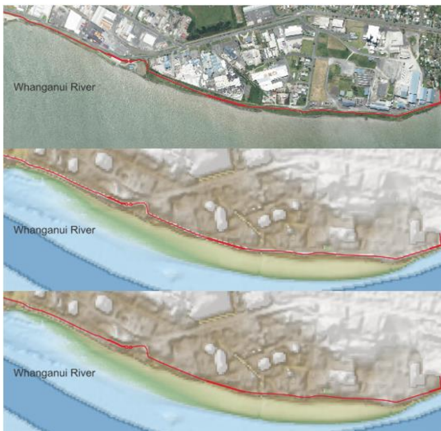
Figure 2-8: DEM for the upper bank of the Whanganui River mouth. Top panel: Aerial photo of the area with the location of the stopbanks highlighted as a red line; Middle panel: DEM with enforced stopbanks for the stopbanks-up configuration, Bottom panel: DEM with removed stopbanks for the stopbanks-down configuration.
