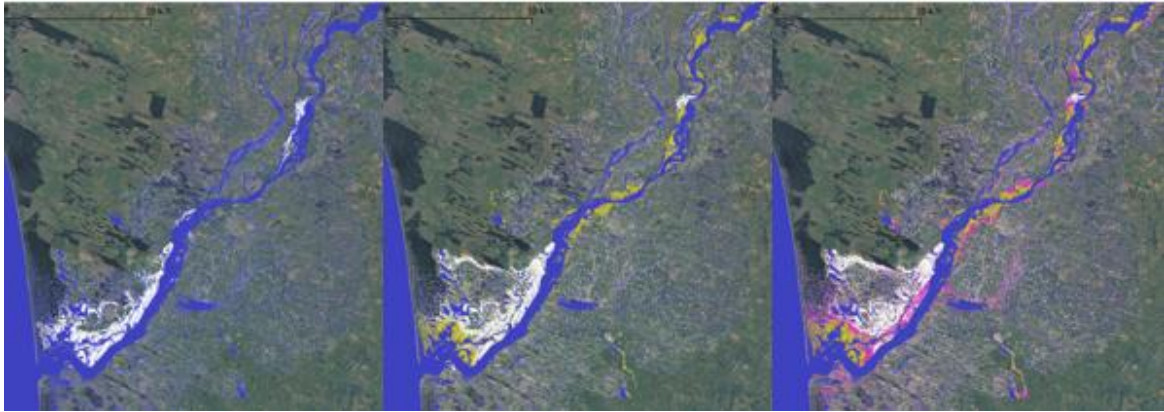
Figure 3-4: Flood extent with stopbank and without stopbanks for the lower Rangitikei area. Left: 20-year ARI in current climate conditions with (blue) and without stopbanks (white). Centre: adding to the left map a 200-year ARI in current climate conditions with (yellow) and without stopbanks (white). Right: adding to the centre map a 200-year ARI + 3°C of climate change warming with (purple) and without (white) stopbanks.
