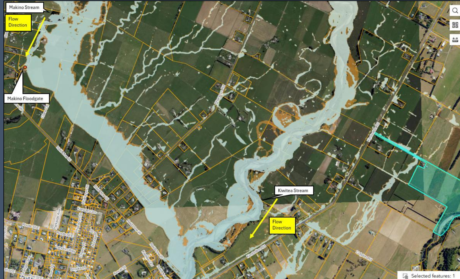
Reid Line Spillway Flood extents for 1 in 200-year (blue) and 1 in 500-year (orange) event (including climate change)
