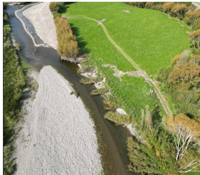
Mahoney's Farm tied-tree work. Pole planting and channel widening.
