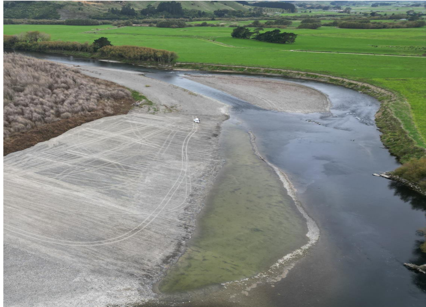
Beach ripping & channel widening, Oxbow Farm – Manawatū River.
