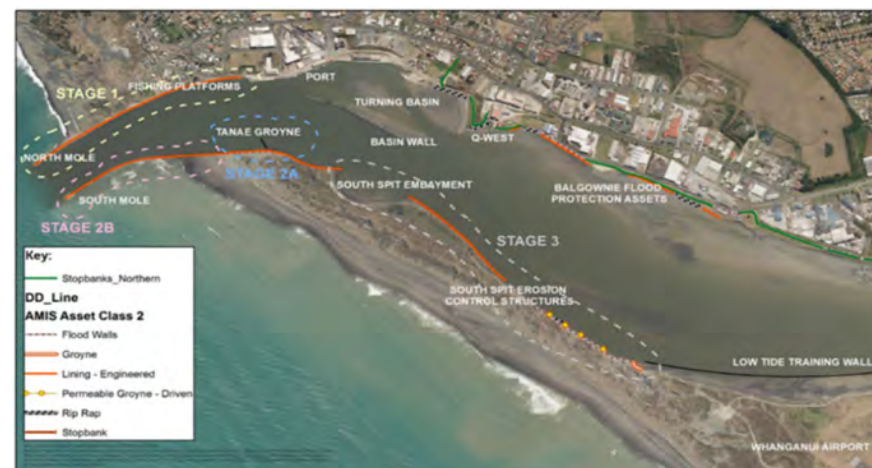
Figure 20: Te Pūwaha project stages and assets overview.
