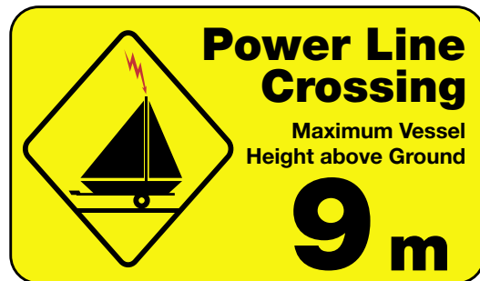
SIGN INSTALLED ON RAMPS ACCESSING WATERWAYS WHERE THERE ARE OVERHEAD LINE CROSSINGS
