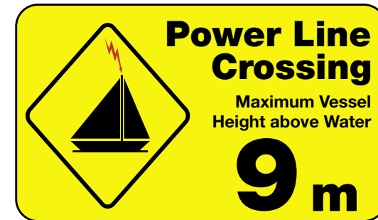
SIGN INSTALLED ON EACH SIDE OF AN OVERHEAD LINE CROSSING
