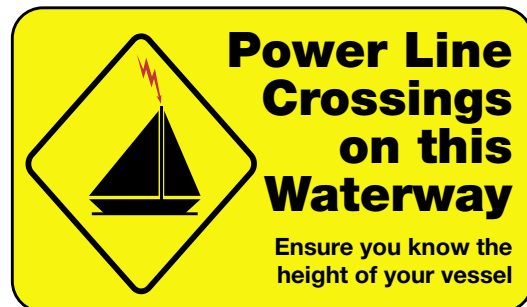
SIGN INSTALLED ON RAMPS ACCESSING WATERWAYS WHERE THERE ARE OVERHEAD LINE CROSSINGS
