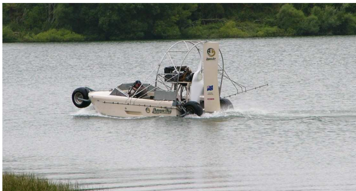
Figure 45. Spraying alum onto the surface of Lake Okaro. The air boat was fitted with GPS navigation to control where the spray was applied.
