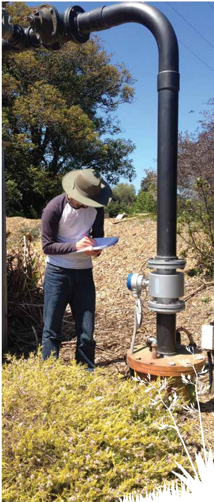
Measuring reference levels for groundwater height
