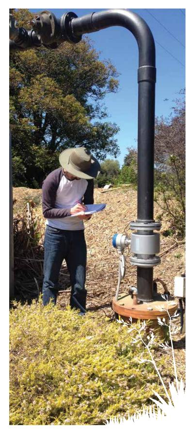
Measuring reference levels for groundwater height
