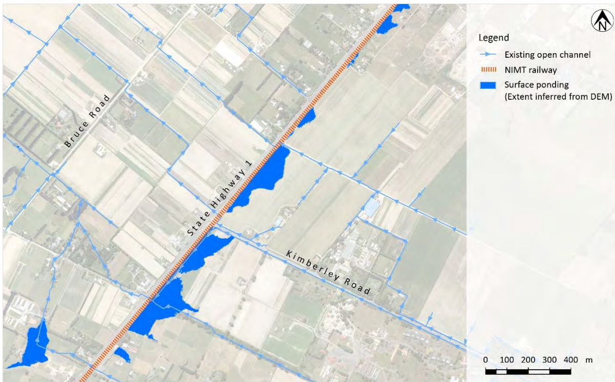
Figure 16. Example of inferred maximum surface ponding against the railway embankment
