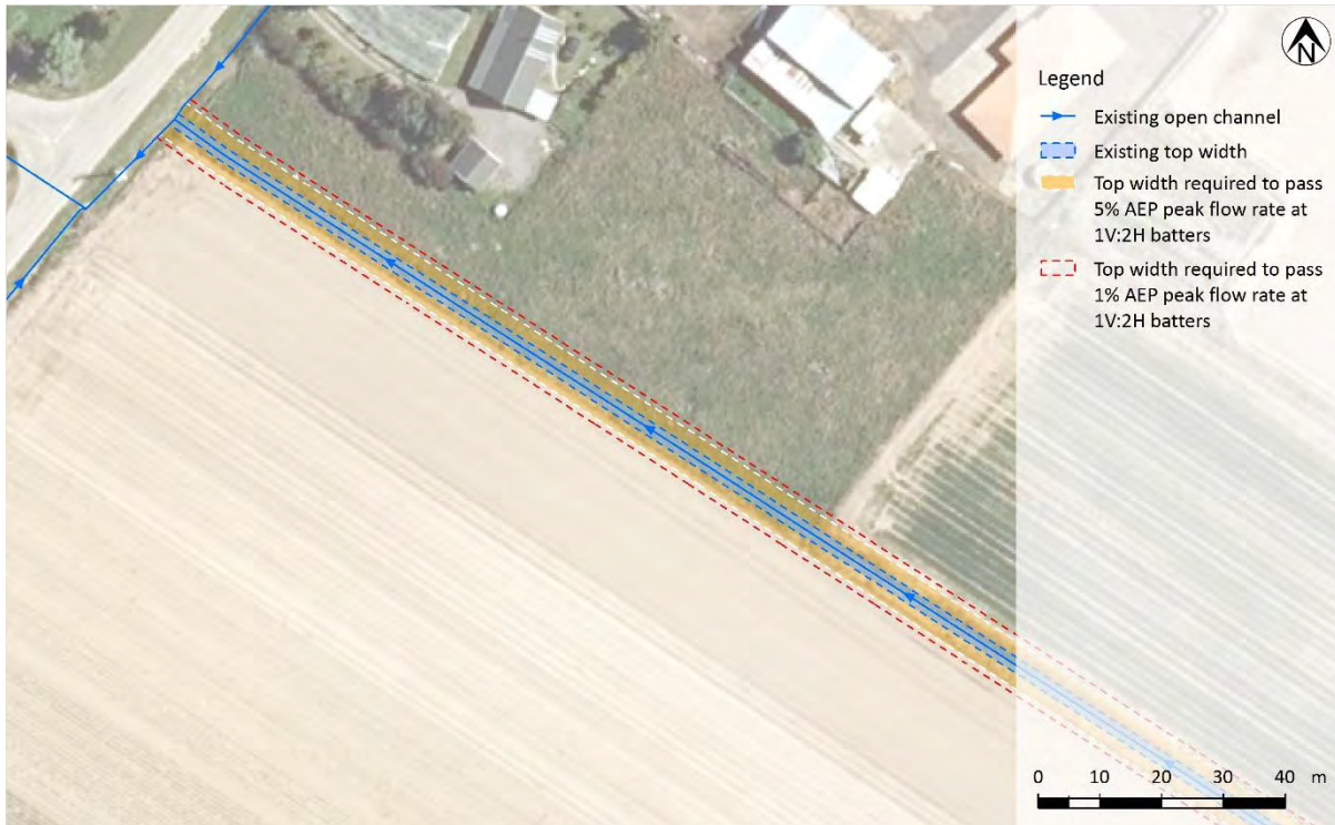
Figure 22. Change in land area requirement for channels of variable bed width and side slope (Drain 3 XS1735)
