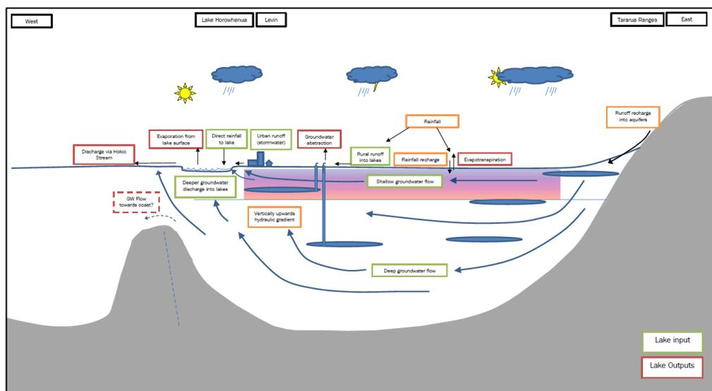
**Figure 5: Conceptual cross section (blue ovals represent silty lenses within the strata)**
