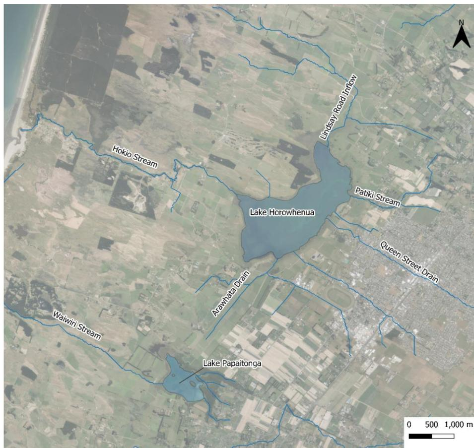
**Figure 11: Lake Horowhenua surface water inflows and outflows**
