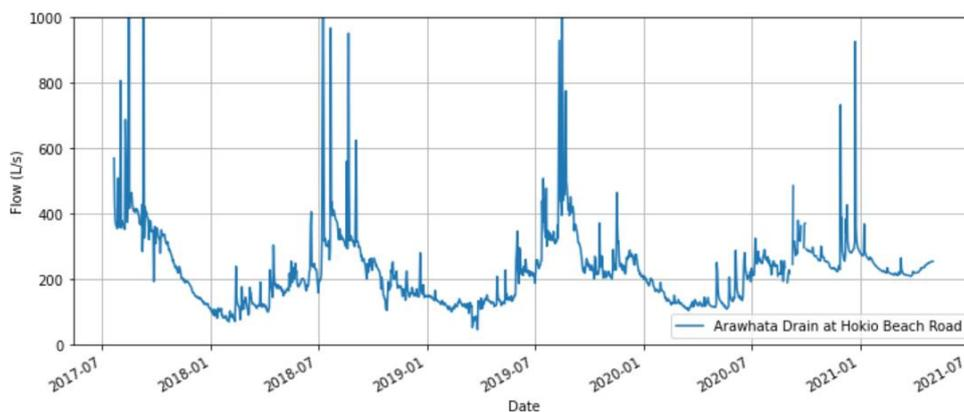
**Figure 12: Flows in the Arawhata Drain at Hokio Beach Road**
