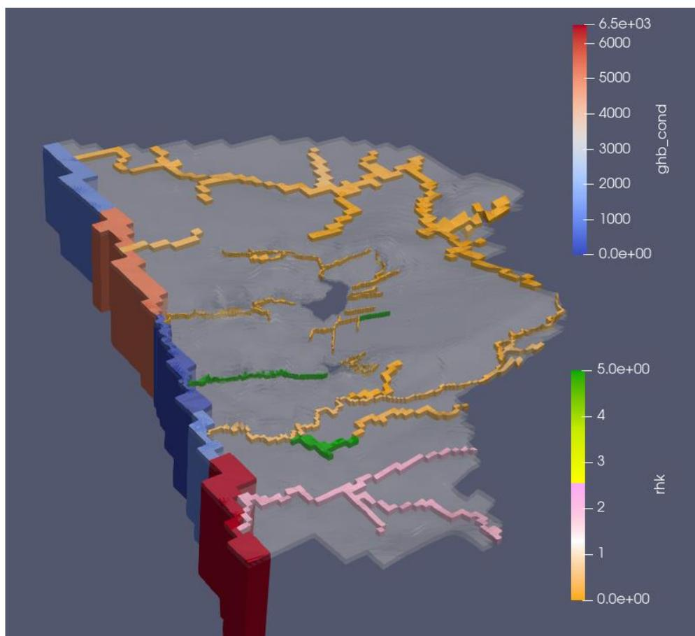
**Figure 20: Boundary conductances (ghb = general head boundaries, rhc = river hydraulic conductivity)**
