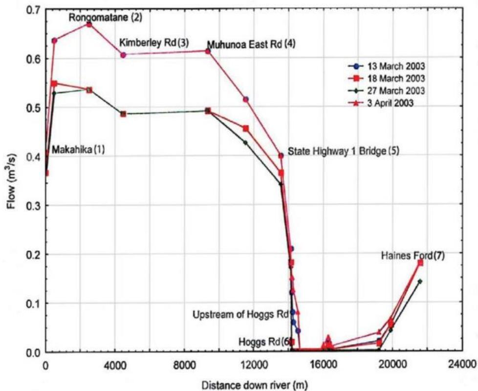
Figure 10: Ōhau River gaining and losing reaches
