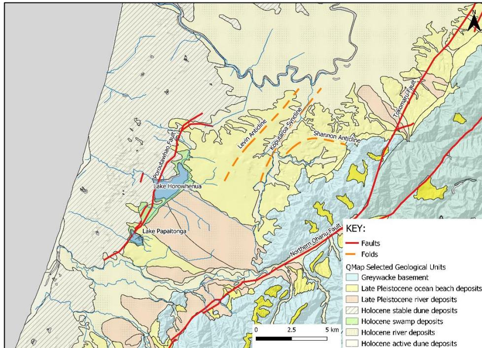
**Figure 2: Geological map of the model area (after Begg and Johnston, 2000)**
