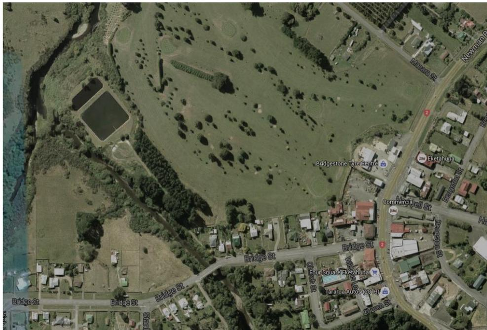
14. The treatment plant serves around 450 people (2013 census) and currently consists of two oxidation ponds discharging to the Makakahi River. The plant is gravity fed. Pond 1 is a facultative oxidation pond with mechanical aeration and Pond 2 is a maturation pond. Anaerobic biological activity will occur in the sludge layer at the bottom of the ponds and potentially at lower levels in the water in the facultative pond.
