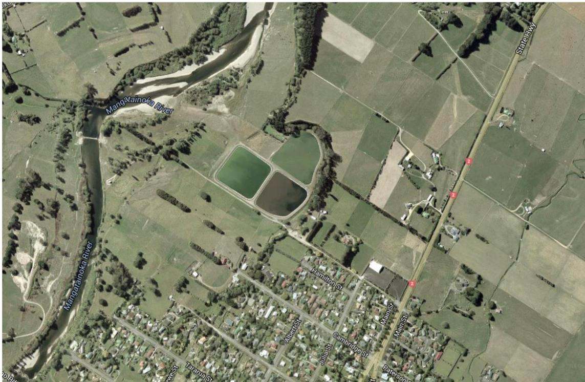
14. The Pahiataua Wastewater Treatment Plant serves around 2400 people (2013 census) and currently consists of three oxidation ponds discharging to the Mangatainoka River via Town Creek. The ponds are facultative oxidation ponds with mechanical aeration in Pond 1 and Pond 2. Anaerobic biological activity will occur in the sludge and at lower levels in the water in the ponds.
