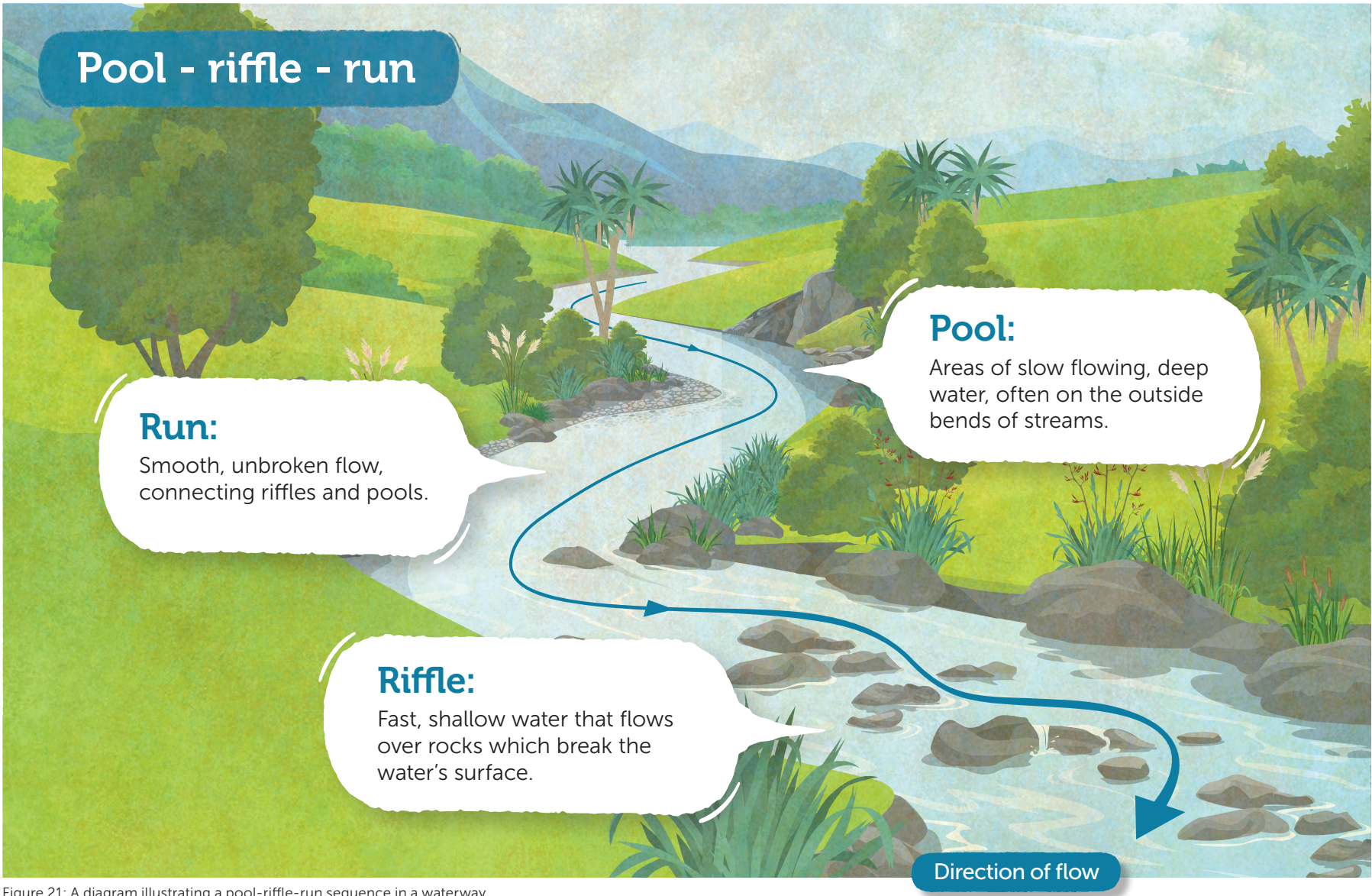
Figure 21: A diagram illustrating a pool-riffle-run sequence in a waterway
