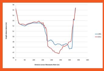
*Figure 27:* Cross-sectional view of temporal changes in mean bed level in the Manawatu River, at Ashhurst Bridge
