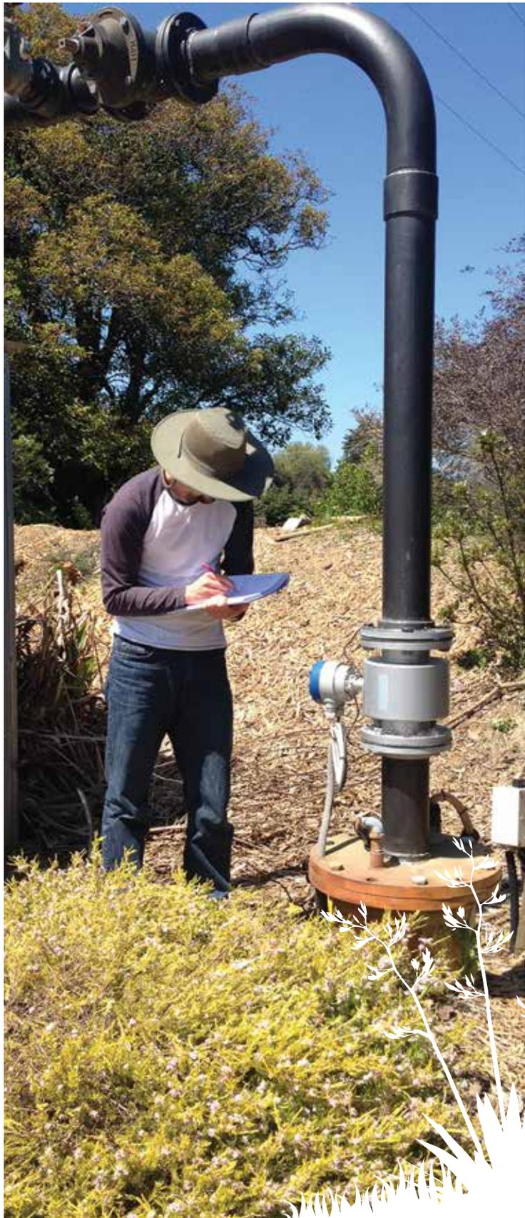
Measuring reference levels for groundwater height
