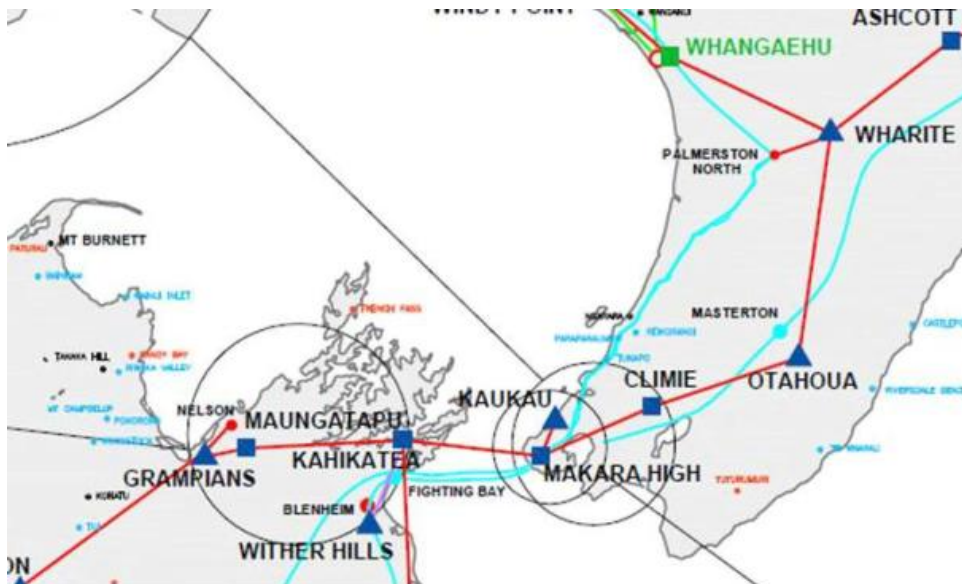
Figure 8.17: Kordia services in the Lower North Island. Red line: microwave linking, Light blue: Fibre, Blue triangles/ squares: High sites, Red dots: Inner-city interconnect sites (Manawatū-Wanganui Emergency Management Group, 2016).
