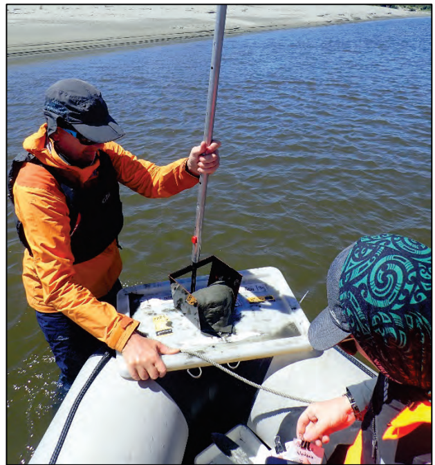
Hoe sampler, collecting sediment by wading
