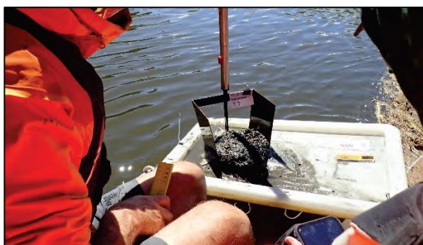
Sediment collected with hoe sampler
