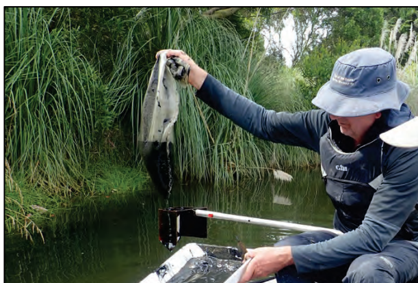
Sediment sample in 0.5mm sieve bag prior to sieving
