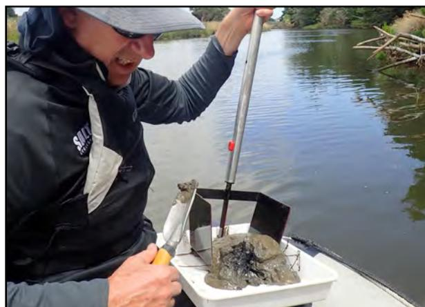
A modified benthic hoe was used to collect sediment from water <3m deep
