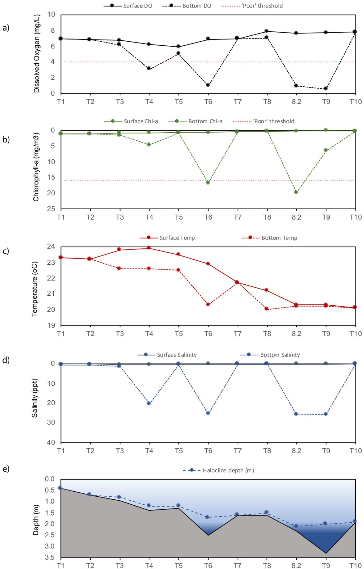
Fig. 11. Water quality measurements collected in Jan 2019 showing surface and bottom water results for: a) dissolved oxygen; b) chlorophyll-a; c) temperature; d) salinity; and e) halocline depth.
