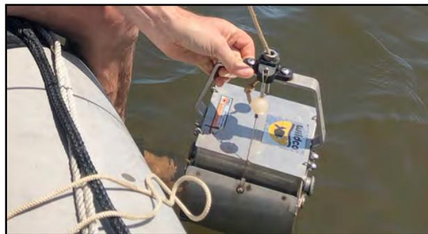
A box core was used to collect sediment in deep water
