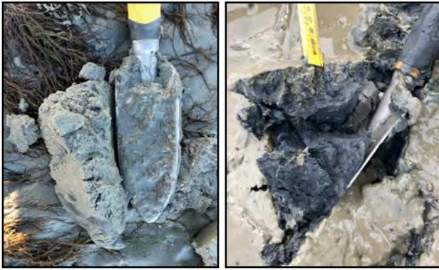
Examples of well oxygenated sandy sediment with aRPD >150mm (left) and poorly oxygenated muddy sediment with aRPD <5mm (right).
