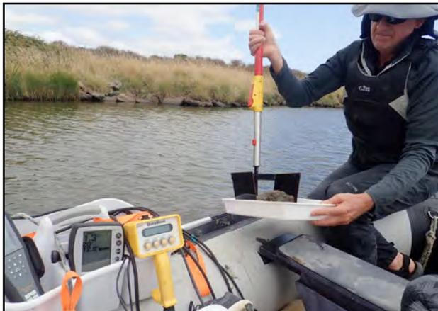
Subtidal sampling used a modified benthic hoe sampler or a box core, and a suite of water quality instruments
