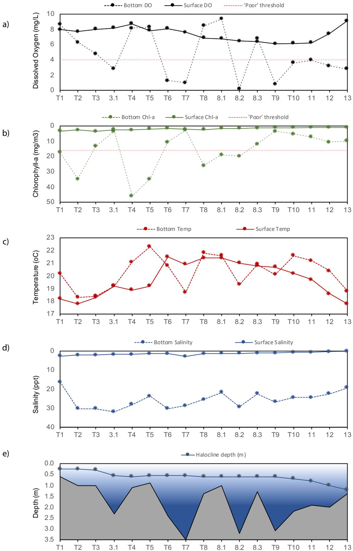
Fig. 12. Water quality measurements collected in Jan 2020 showing surface and bottom water results for: a) dissolved oxygen; b) chlorophyll-a; c) temperature; d) salinity; and e) halocline depth.
