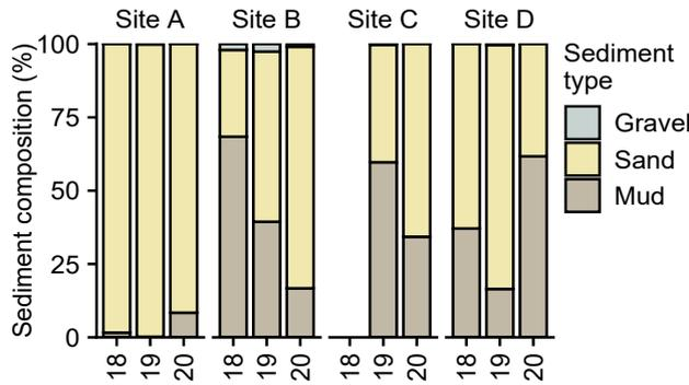
Fig. 14. Sediment particle grain size analysis, showing site-averaged percentage composition of mud (<63µm), sand (<2mm to ≥63µm) and gravel (≥2mm).
