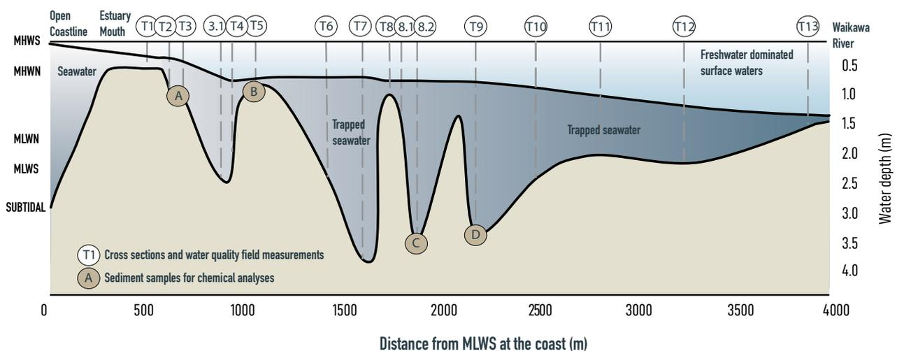
Fig. 10. Simplified longitudinal cross-section of lower Waikawa Estuary showing bed height, sediment sampling locations and location of channel cross-sections.
