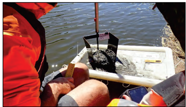
Sediment collected with hoe sampler
