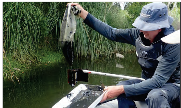
Sediment sample in 0.5mm sieve bag prior to sieving
