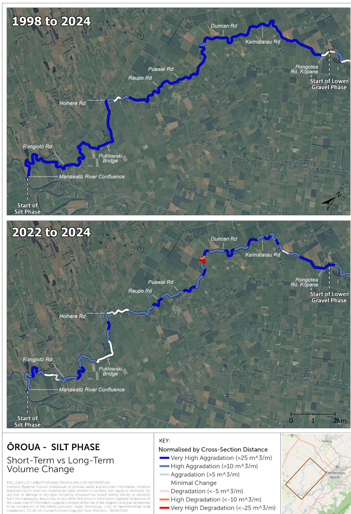
Figure 33 Sediment volume change between 1998 and 2024 compared to 2022 to 2024 for the silt phase of the Ōroua River (using 2022/2024 active channel offsets).
