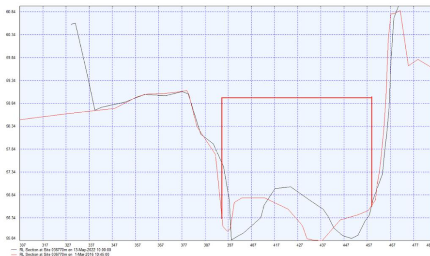
Figure 10 Example Section from the gravel phase with active channel indicated for Men Bed Level calculations. Multiple thread channel sections include both invert. Single thread sections are taken bank to bank or bank to highpoint of lateral bar (King, 2023).
