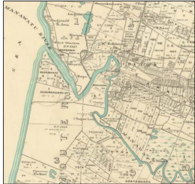
Lands & Survey map showing Manawātū River in 1929 prior to the Whirokino Cut, completed in 1943, that bypassed 7km of the lower river. Sourced from https://www.mapspast.org.nz/
